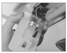
6.16b Interior (courtesy) light pivoted for access to the bulb
